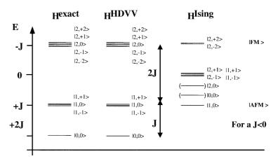
In the case of many magnetic centres it is not always possible to find the eigenfunctions of the HDVV Hamiltonian [22]. This is also the case for periodic systems, where exact solution for HDVV exists for one-dimensional systems only. A common approach to the computation of the magnetic coupling constant for periodic systems is to make use of a simplified version of the HDVV Hamiltonian in which the total spin operators are substituted by the z-component of this operator,
