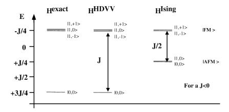
Fig. 2. Energy diagram for the eigenstates of the exact, HDVV and Ising model Hamiltonians for a system of two S=1 interacting spins. States in parentheses indicate that these particular *eigenstates* of the HDVV Hamiltonian are not eigenfunctions of the Ising Hamiltonian, the energy in these cases is just an expectation value
